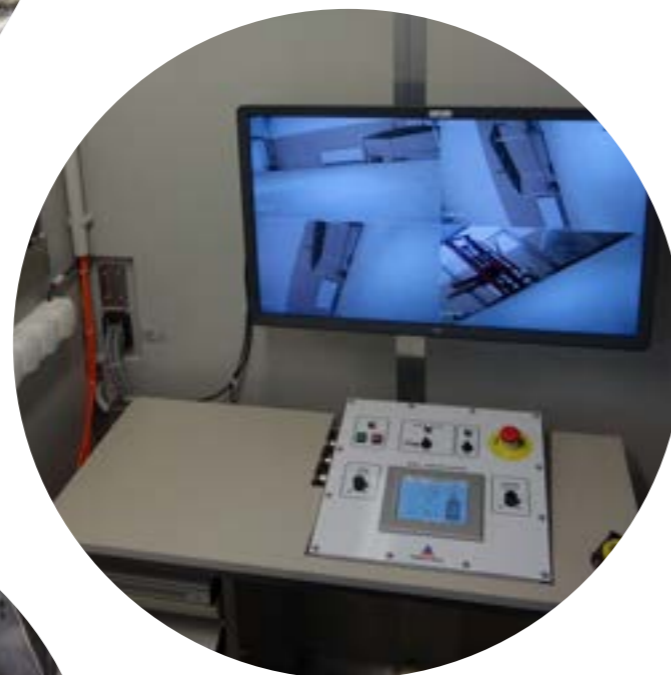
The operator sees every movement of the robot in real time on a high-definition monitor
