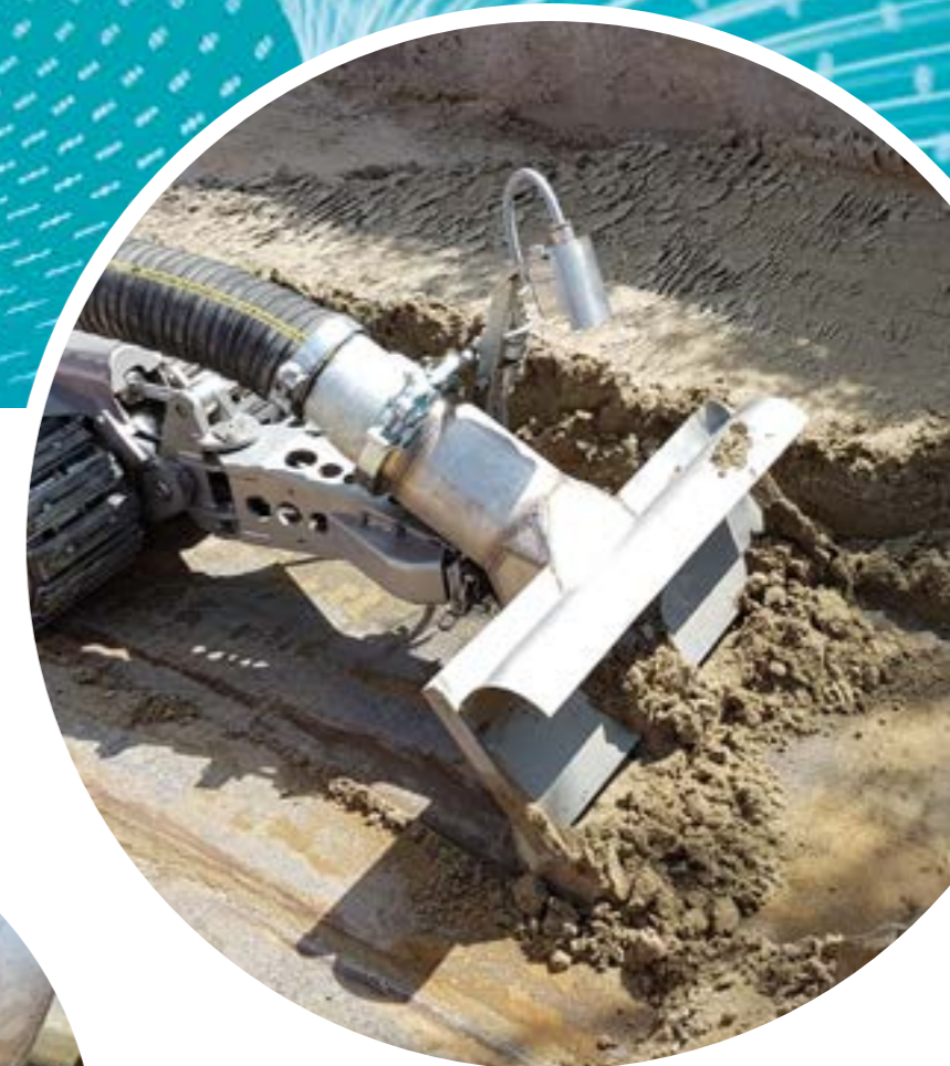
ADEX Robot for rough cleaning of flat-bottom tanks in ATEX Zone 0
